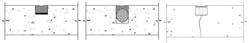
2. The backer rod supports tooling so after installation of material the sealant can be pushed to the bond line with a spatula, ensuring wet-out of the sealant to the substrate.
