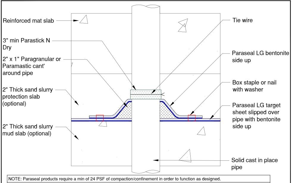
NOTE: Use washer headed nails in the seam areas only as needed. All nails to be located at the seam lap and covered by or driven through a piece of Parastick N Dry.
