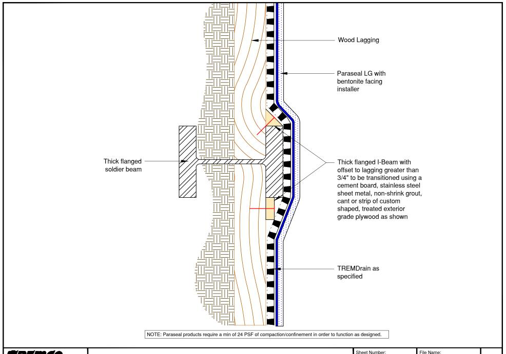
3735 Green Road \* Beachwood, OH 44122 Phone: 866-209-2404 \* Fax: 216-766-5535 Detail: PARASEAL LG TRANSITION AT THICK FLANGED BEAM-PLAN VIEW
