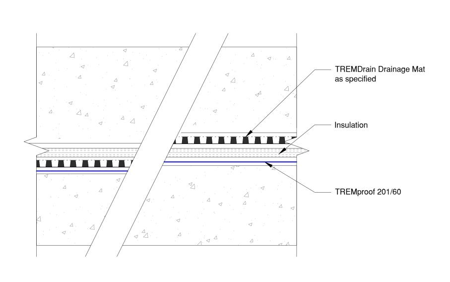
Note: Insulation Should Not be Placed onto Uncured Membrane
